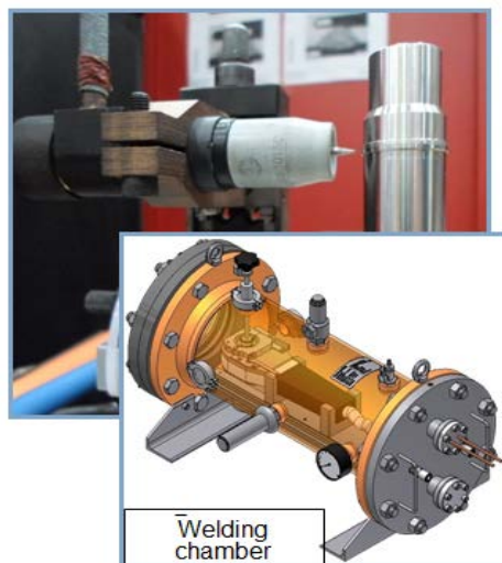
Fig. 8. Qualified welding method and equipment for dry and welded capsule for DFR
